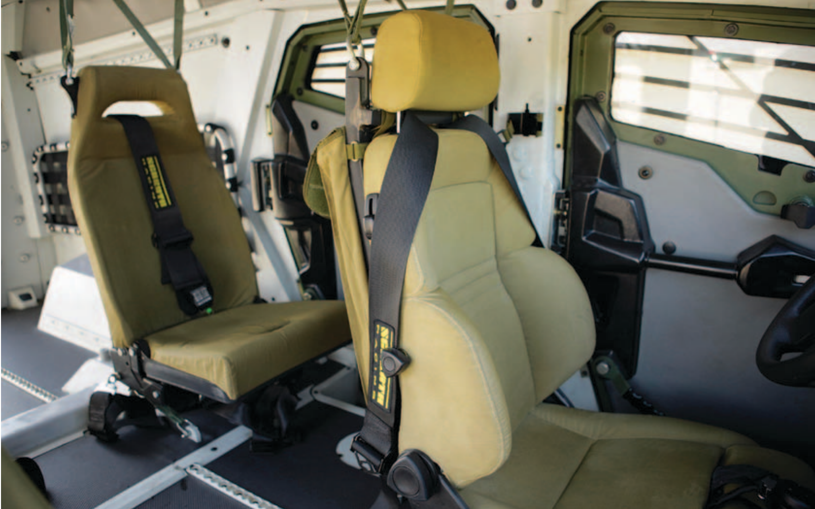
Tactical Protector Vehicle™ interior as configured with suspended seating for four and fold-away rear bench seats.
